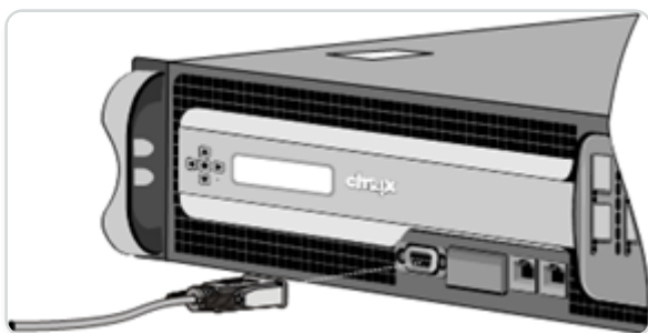
Figure 9. Insert a console cable
