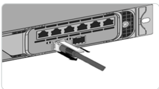
Figure 9. Remove a DAC from the 10G port
