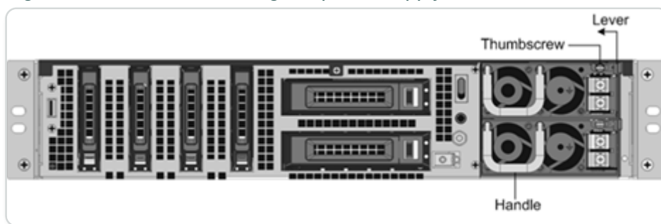
Figure 2. Remove the existing DC power supply
