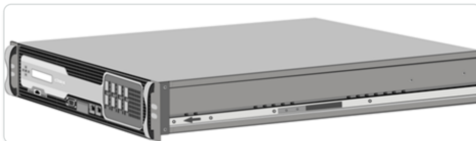
Figure 1. Attach inner rails
